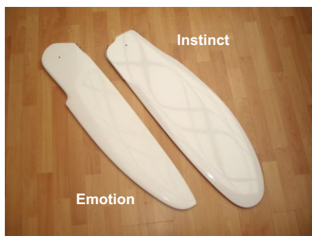
42015 Rudder blade - Instinct 42115 Rudder blade - Emotion Fibreglass - epoxi, Colour: White
